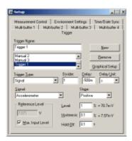
30. Now that the trigger has been configured, it is now necessary to configure the FFT analyser. Right click 'FFT Analyser' and select properties. This brings up the configuration for the FFT Analyser. Using this window it is possible to control a number of aspects of the FFT Analyser, including the resolution or number of lines used by the analysis, the frequency span of the analysis, type of averaging used and triggers can be applied.
