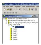
13. To make the changes that have been made to the 'Configuration Organiser' applicable to other windows it is necessary to click the 'Activate Template' button or press F2.
