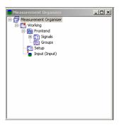
15. It is now required to setup signal groups. Signal groups are required because they the analysers that will be used shortly to accept multiple signals. It is only possible to feed a signal into a Pulse Analyser by grouping it first. This step may seem a bit pointless when there is only one signal, but the need for this step will become clear when multiple signals are being used. In this case, right click 'Groups' and select 'New Group'.
