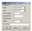
5. Enter a 'Nom. Sensitivity' and 'Sensitivity Unit' for this combination. When a 2635 is used, the sensitivity can be set using the dials on the front of the unit. In this case select a 'Nom. Sensitivity' of 10 and a 'Sensitivity' of 'mV/ms^-2'. The weight of the accelerometer can be found on the calibration sheet provided with all accelerometers. In this case a 4393 Accelerometer weighs 2.4g. A description can be added if desired.
