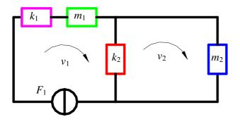
Applying the mesh current method, we can write the equation for the 2 meshes (2-DOF) :
