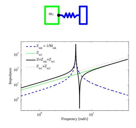
The anti-resonance happens at the frequency where the  $Z_{mk} = Z_{m_l}$ ,
