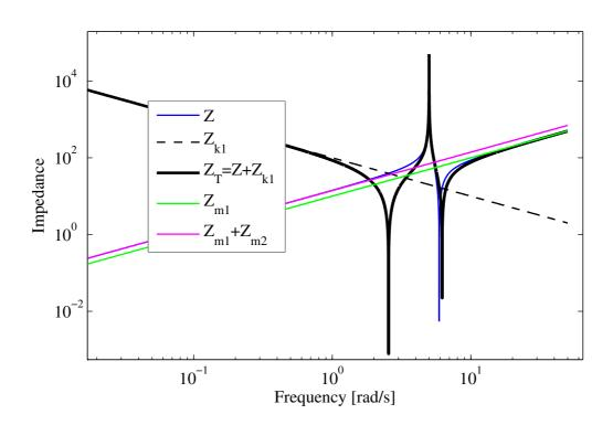
The first minimum in the impedance happens when  $Z_{m_1} + Z_{m_2} \simeq Z_{k_1}$ ,  $j\omega(m_1 + m_2) \simeq \frac{k_1}{j\omega}$ to get  $\omega \simeq [k_1 / (m_1 + m_2)]^{1/2}$  ( $\omega = 2.67$  rad/s)
